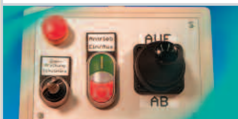
Bottom: Control console with joystick for shift operation as well as for fast manual testing
